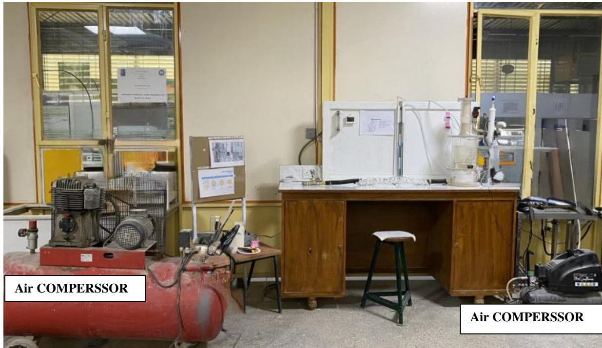
Figure 2a. Experimental setup of Batch fluidized bed granulator
