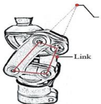
Figure 3. Mechanical passive knee joints: (Polycentric Knee with 4-bar linkage mechanism) [14]
