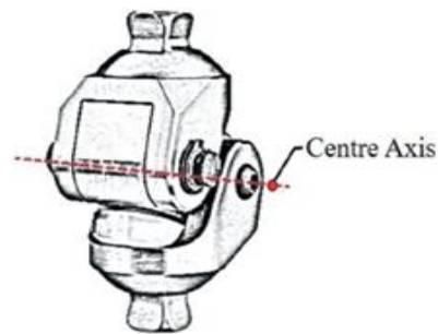
Figure 3. (Mechanical passive knee joints) Single-axis [14]
