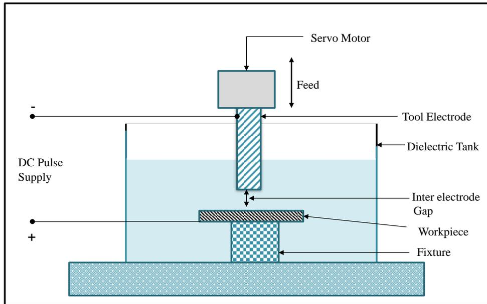
Figure 1. Schematic of an Electric Discharge Machining (EDM) machine tool
