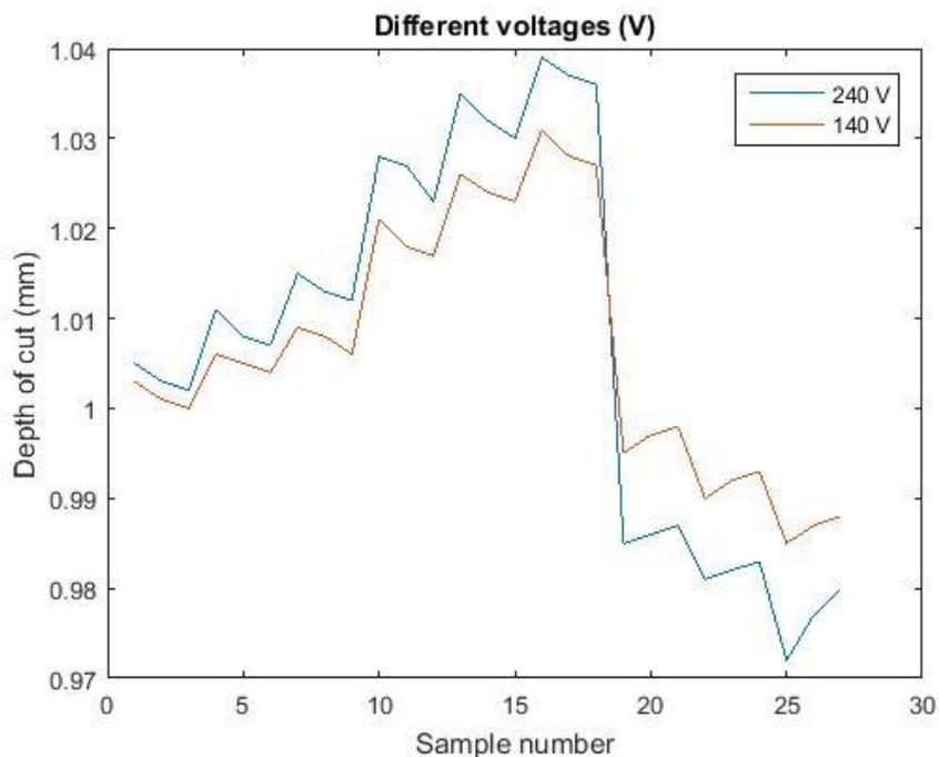
Figure 4: Relationship between the Depth of Cut and sample number for both voltages (140. 240V).
