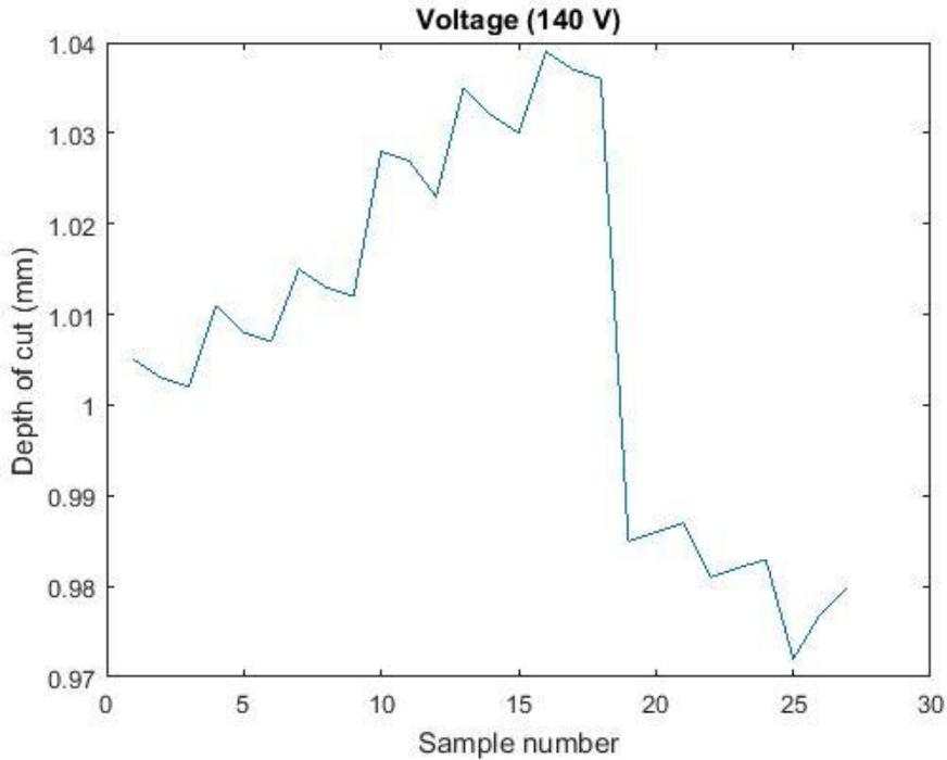
Figure 2: Relationship between the Depth of Cut and sample number for 27 samples and 140V
