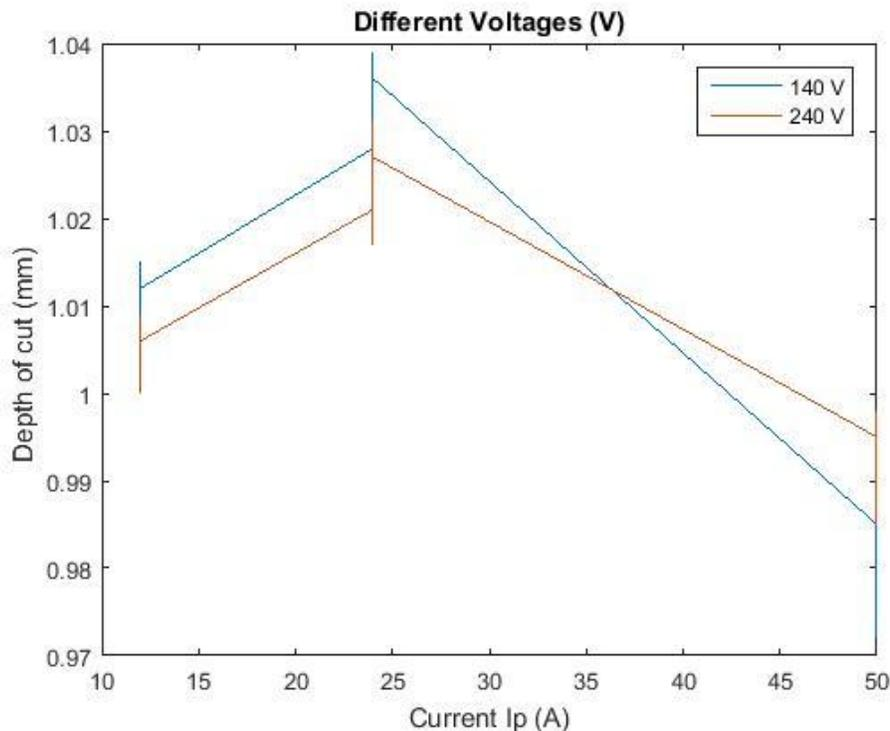
Figure 5: Relationship between the Depth of Cut and current ( $I_p$ ) for both voltages (140 V. 240V).
