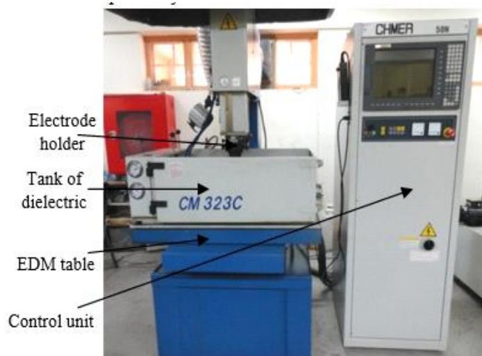
Figure 3. A CM323C CNC EDM machine was employed for the experiments conducted in this work. The work material used in this study is high speed steel AISI M2 with nine specimens dimensions (60×45×3 mm). The chemical composition and mechanical and physical properties of the work material is given in Table 1 and Table 2 respectively.
