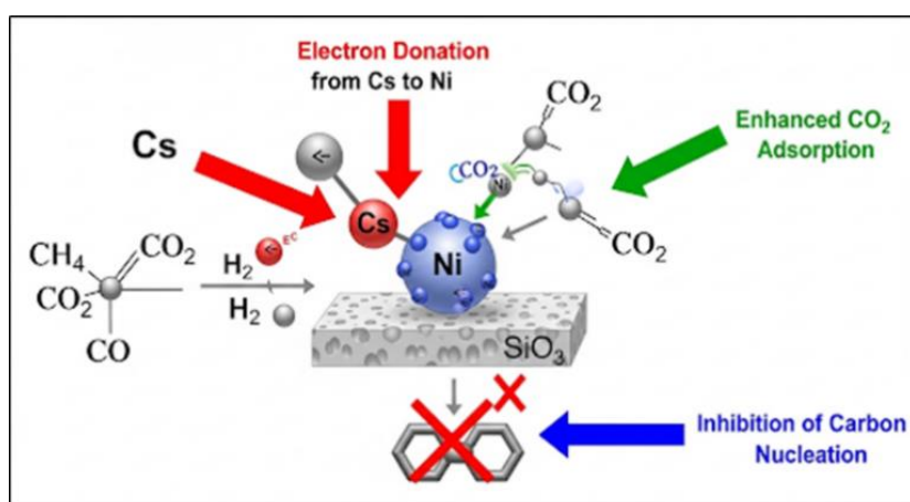
Figure 2. Schematic of the mechanistic pathways of Cs-promoted Ni catalysts in DRM.
