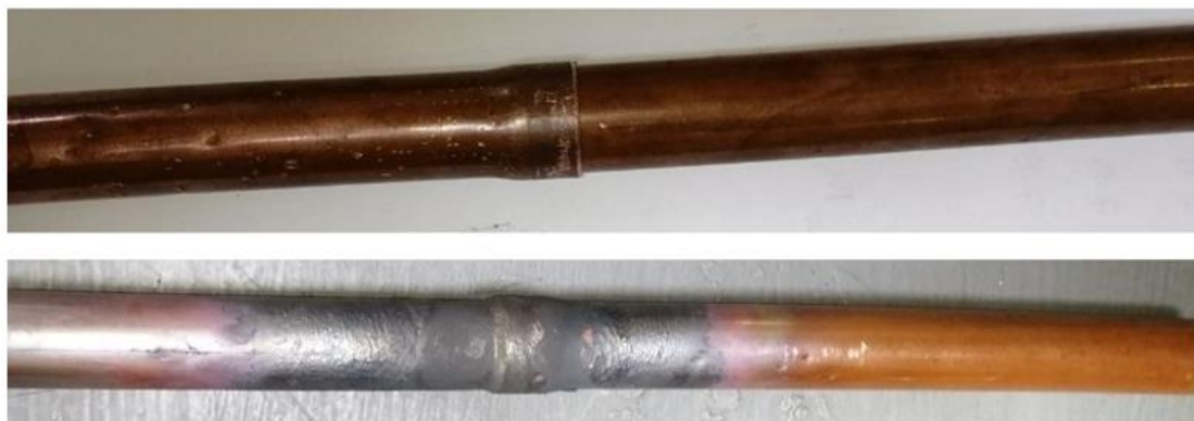
Figure 1. Overlap design of weld joint
