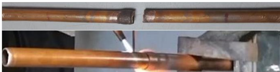
Figure 2. Fracture of welded specimen under tension
