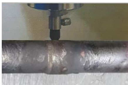
Figure 3. Specimen under Hardness testing
