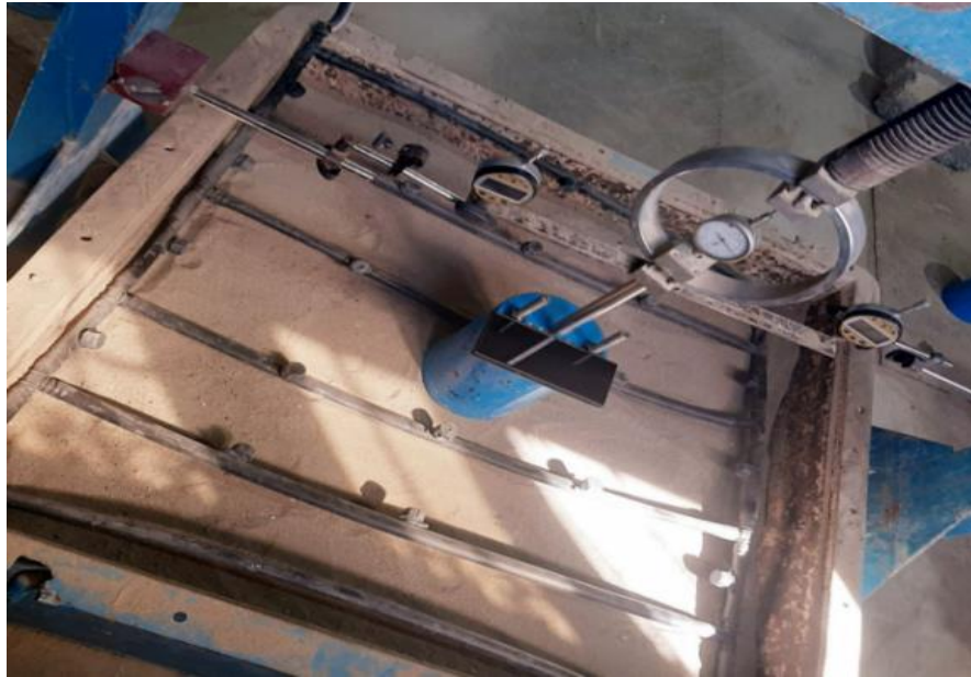
Figure 6. The mechanism used for applying load and measuring load and settlement.
