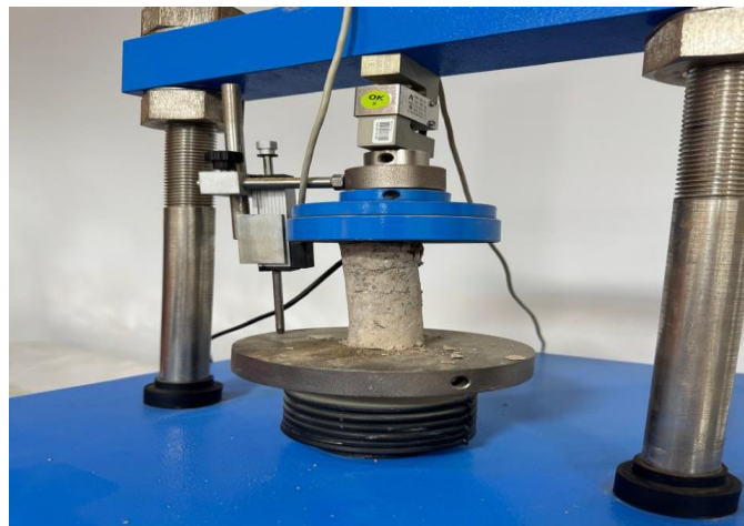
Figure 5. The model examined by the unconfined compression device.
