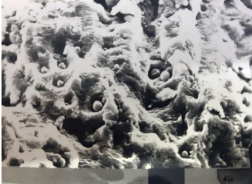
Figure 7. Spherical MnS inclusions
