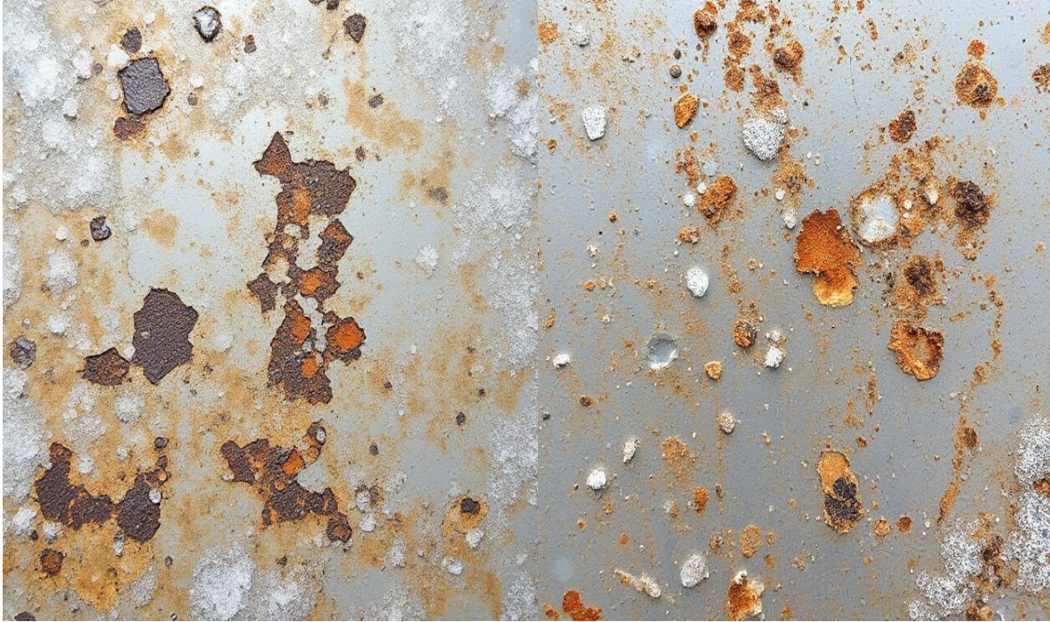
Figures 4 Corrosion Patterns of Aluminum Alloys in Marine and Industrial Environments
