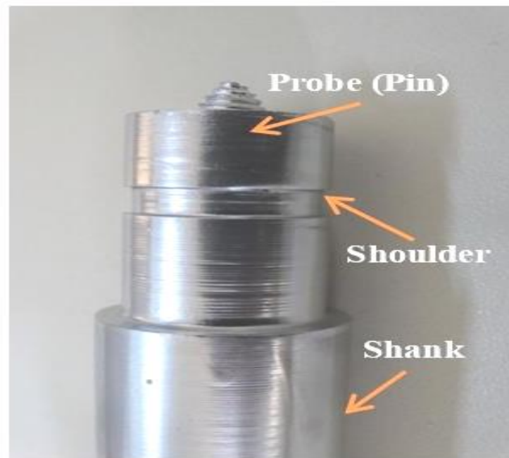
Figure 2: Photograph of FSW Tool Showing Its Different Parts
